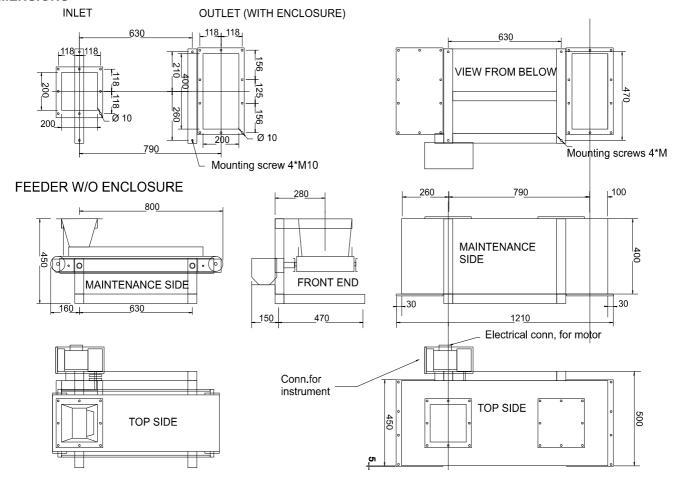
Cut-out according to DIN 24 193-2
