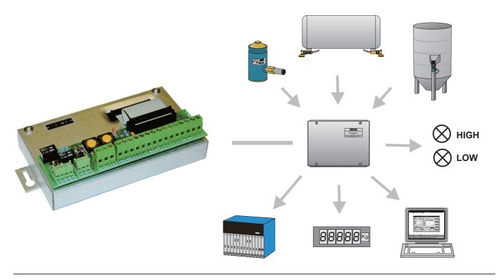
The S-E-G system W3 transmitter is used for analog load cell to digital conversion, level control and weight/signal monitoring via RS485 serial communication, or 4-20 mA analog output current signal. The load is sensed by Strain gauge loadcells selected for the desired load range. The transmitter is also available in stainless field enclosure for use in harsh industrial environments requiring heavy duty equipment with high reliability and IP65 protection.
